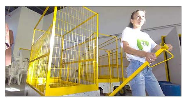
**All over Brazil:** electric push-carts **c**an transport more than 300 kg load. Its autonomy is 4-5 hours, which gives an average of 25 km / day continuous motion.
